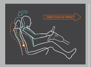
RESPONSIVE SEATING Whiplash Injury Lessening<sup>15</sup> front seatbacks are designed to push backward, allowing occupants to sink into their seats. This can dramatically reduce head movement and the severity of whiplash injury.
