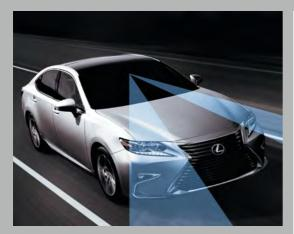
**LANE DEPARTURE ALERT** Lane Departure Alert<sup>25</sup> intelligently monitors the road ahead and provides an audible warning along with steering wheel vibration if your vehicle begins to drift from its current lane without signalling intent.
