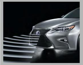
**DYNAMIC RADAR CRUISE CONTROL AND PRE-COLLISION SYSTEM** Using a radar sensor in the vehicle, Dynamic Radar Cruise Control<sup>7</sup> helps you maintain a safe distance from other vehicles by automatically adjusting throttle or braking when cars ahead slow down. In situations where the Pre-collision System <sup>6</sup> senses a high probability of collision, it will issue an audible warning.
