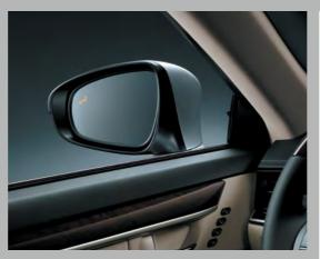
**BLIND SPOT MONITOR** The 2017 ES offers the Blind Spot Monitor System,<sup>6</sup> which uses radar sensors to help alert you to vehicles in your blind spots, allowing you to keep your focus on the road ahead.
