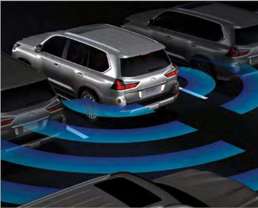
**THE SCIENCE OF SAFETY** You'll stay doubly protected with the standard Blind Spot Monitor,<sup>28</sup> which is rear-mounted radar that detects vehicles you can't see and lights an alert icon in your side mirror. Plus, Rear Cross-Traffic Alert<sup>29</sup> uses quasi-millimetre wave radar to help detect approaching vehicles and warns the driver via audio alert and side-mirror indicators.
