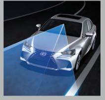
LANE DEPARTURE ALERT<sup>12</sup> While your eyes are set on the road ahead, a camera works as a sensor to recognize lane markings around you, alerting when the vehicle deviates from its lane.
