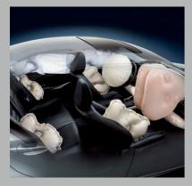
**TEN STANDARD AIRBAGS** The comprehensive safety of the IS ensures every part of the cabin is covered, with side curtain and knee airbags for the driver and front seat passenger and rear outboard-seat side airbags.
