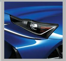
**AUTOMATIC HIGH BEAM**<sup>18</sup> Light your way as necessary, thanks to an in-vehicle camera sensor that assesses the brightness of streetights, the lights of oncoming and preceding vehicles, and automatically turns the high beams on or off as conditions dictate.
