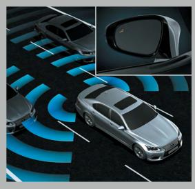
**BLIND SPOT MONITOR** The 2017 LS offers the Blind Spot Monitor System, which uses radar sensors to help alert you to vehicles in your blind spots, allowing you to keep your focus on the road ahead.
