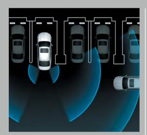
**REAR CROSS-TRAFFIC ALERT** When in reverse. the available Rear Cross-Traffic Alert System<sup>17</sup> uses quasi-millimetre wave radar to help detect any vehicles approaching behind the LS and warns the driver via audio alert and side-mirror indicators.
