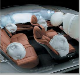
10-AIRBAG SYSTEM Standard airbags include driver and passenger knee airbags, front seat-mounted side airbags, front and rear side-curtain airbags and rear seat side airbags.<sup>19</sup> In addition, front seats are designed to help decrease the severity of whiplash-type injuries in certain rear collisions.
