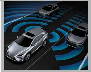
PRECISION SENSORS The 2017 NX offers rearmounted radars that detect the vehicles you can't see, while an alert icon appears in your side mirror.8 And when you're reversing, Rear Cross-Traffic Alert<sup>4</sup> detects and notifies if a vehicle is approaching while you back up.
