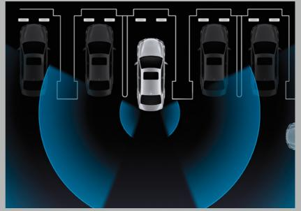
**REAR CROSS-TRAFFIC ALERT** Standard on the RC 350 and available on the RC 300, Rear Cross-Traffic Alert<sup>4</sup> offers peace of mind when your focus is directed behind you. The system uses quasi-millimetre wave radar to help detect approaching vehicles as you back up, warning you through an audio alert and side-mirror indicators.
