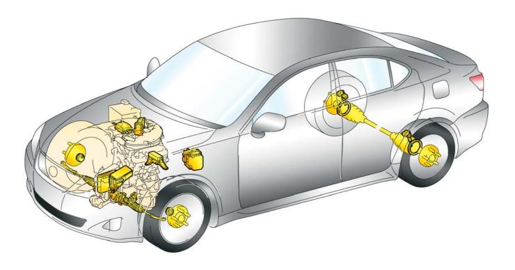
This system cuts engine power in case of simultaneous application of both the accelerator and brake pedals. This system works at speeds of 10 km/h or greater or if the throttle opening is at a value resulting in high engine output.
