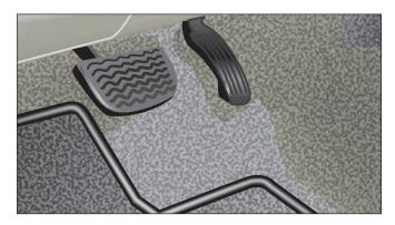
Check the pedal operation by fully depressing the pedal to ensure the floor mat does not intefere with it. When testing, make sure the vehicle is off, in 'Park' (for automatic transmission models) and the parking brake is on.
